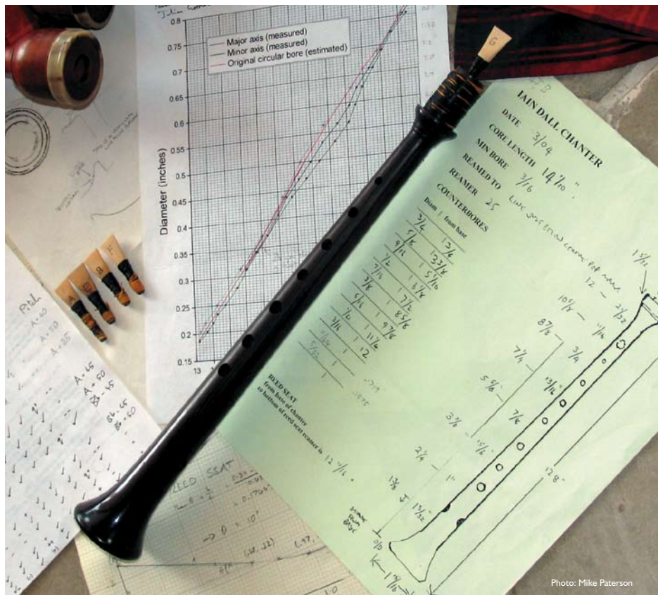
THIS reproduction of Iain Dall's late-17th century chanter was made by Julian Goodacre of Peebles, in collaboration with piper and piping scholar Barnaby Brown. It rests on documents relating to the original measurements and the extrapolations that were made to correct distortions wrought by time on the original chanter, which was carefully preserved by Iain Dall's descendants in Nova Scotia, Canada.
